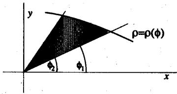
$$2) \quad D : \left\{ \begin{array}{l} \phi_1 \leq \phi \leq \phi_2 \\ \rho = \rho(\phi) \end{array} \right\}$$
