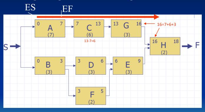
Early Starts and Early finishes dates are calculated by means of Forward Pass
