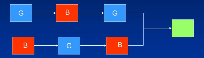
In order to start **B** in the upper branch, you have to finish **G** and also **B** in the lower branch. The probability, that **B** start in time is 50 % worse, than it was shown on the previous slide.
