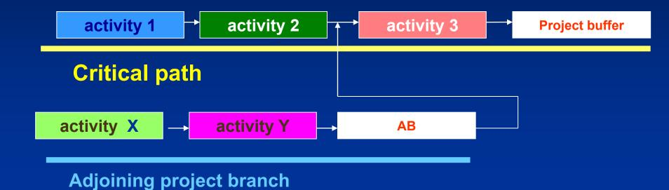
Buffer serves as a safety tool to accumulate reasons of expected and unexpected delays
