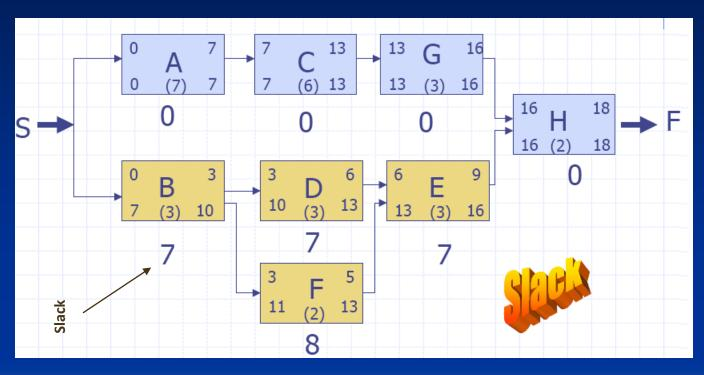
Free Float: Amount of time a single task can be delayed without delaying the early start of any successor task =LS-ES or LF-EF
