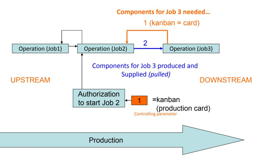
The number of cards in the system determines the WIP levels in the plant
