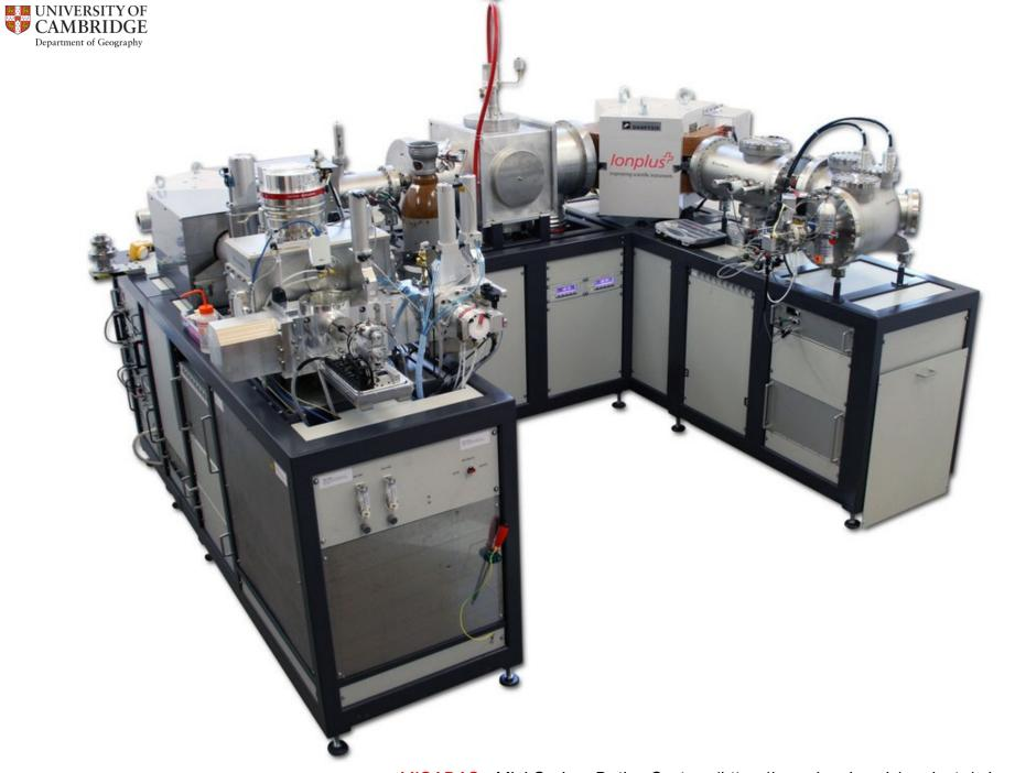
MICADAS - Mini Carbon Dating System (https://www.ionplus.ch/products/micadas/)
