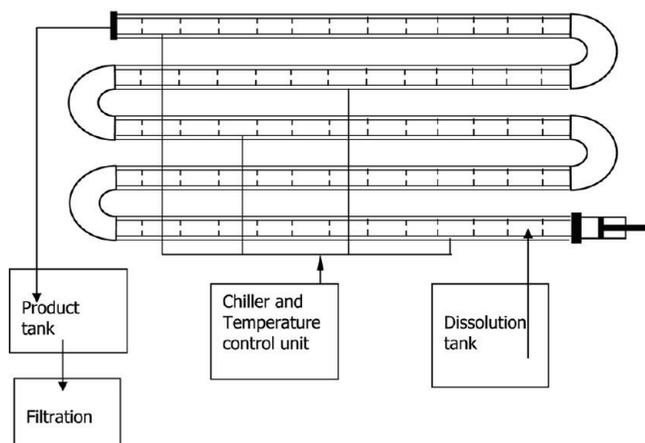
**Figure 2.** Continuous oscillatory baffled crystallizer.
