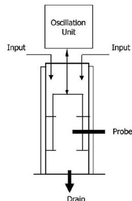
**Figure 3.** The setup of batch OBC.
