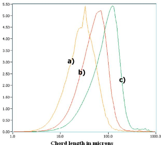
**Figure 6.** SEM of crystals and the corresponding crystal chord size distributions under three experimental conditions. (a) 1 °C/min with 3 baffles; (b) 1 °C/min with two baffles; (c) 0.25 °C/min with two baffles (4 Hz and 40 mm), (4 Hz and 40 mm), (4 Hz and 20 mm).
