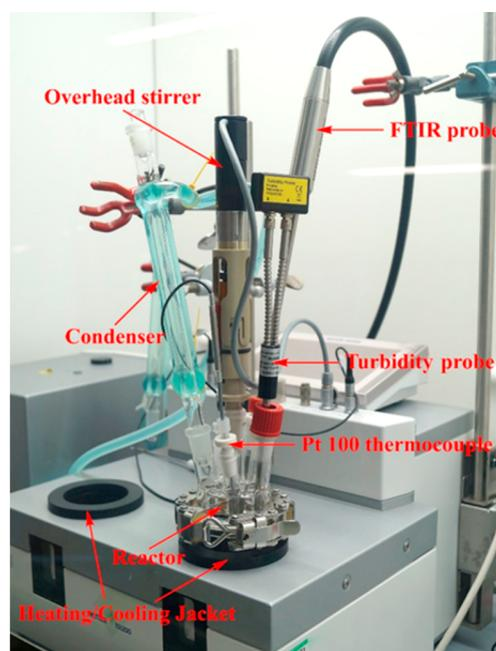
Figure 3. Experimental setup used for induction time and crystallization experiments.
