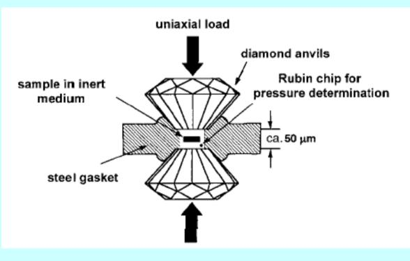
pressure transmitting medium: solid Ar, N<sub>2</sub>, O<sub>2</sub>,
