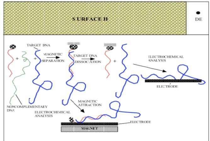
With spherical magnetic beads non-specific binding of NAs is minimized. 20 microL of the bead suspension gives 3 to 7 cm<sup>2</sup> area. Beads can be incorporated into microfluidic systems and chips
