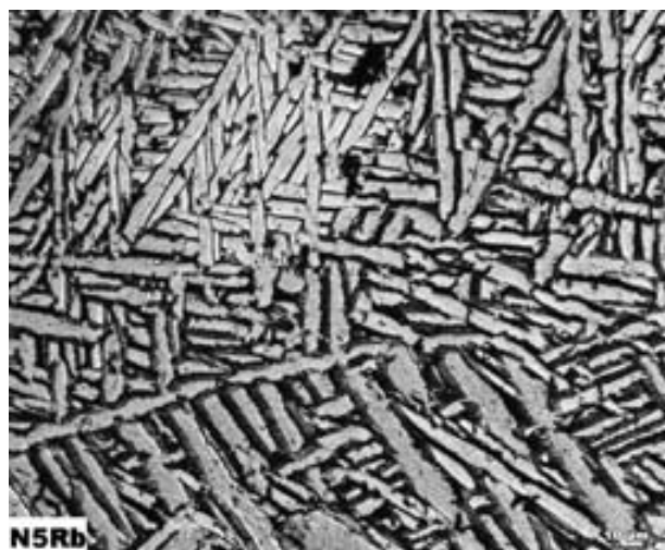
Figure 1 Microstructure of Ti6Al7Nb alloy after casting (left) and Ti6Al10Nb cooled 10 min at 850 °C/10 (right).
