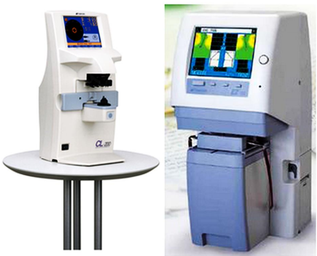
Picture 6.1: Digital automated lensmeter (Benes et al. 2010).
