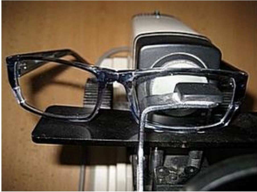
Picture 6.2: Right spectacles' position in the lensmeter (Benes et al. 2010).
