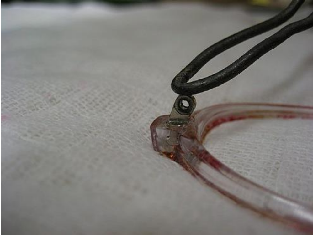
Picture 13.1: Replacement of the melted side connection (Benes et al. 2010).
