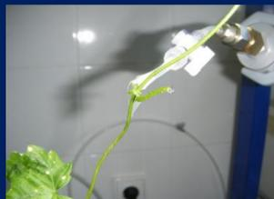
The pressurization chamber in working set up; connection between plant and the sensing unit and the droplet to be extracted.
