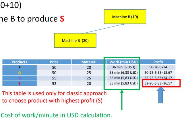
Calculated time of work includes both machines (A and B)
