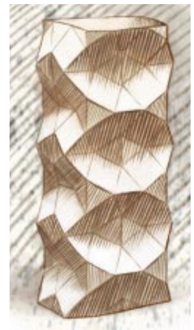
BUCKLED CYLINDERS correspond to red, green and orange foldings (below).
