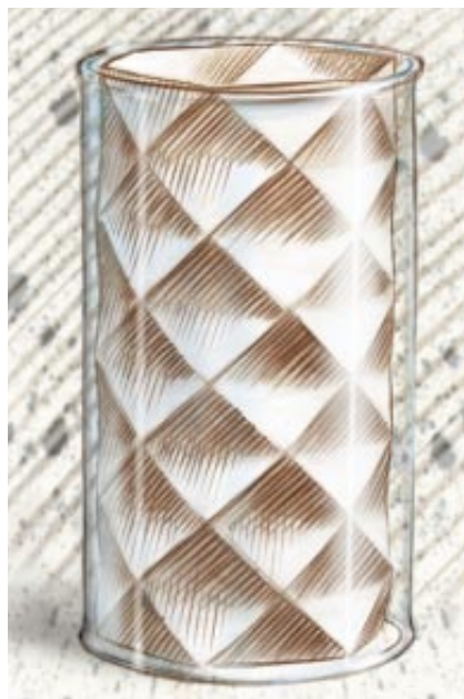
YOSHIMURA PATTERN corresponds to the primary mode of buckling of a cylinder.
