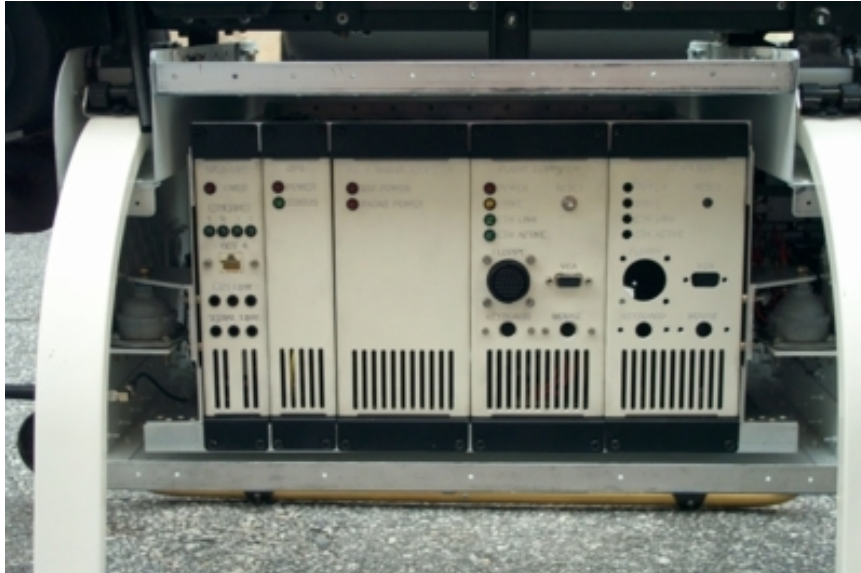
Figure 4: Shock-mounted avionics rack on the airframe, front outer box cover removed, from left to right: Data Link Module, GPS module, IMU/Radar Module, Flight Computer Module, Auxiliary Module (uncompleted)
