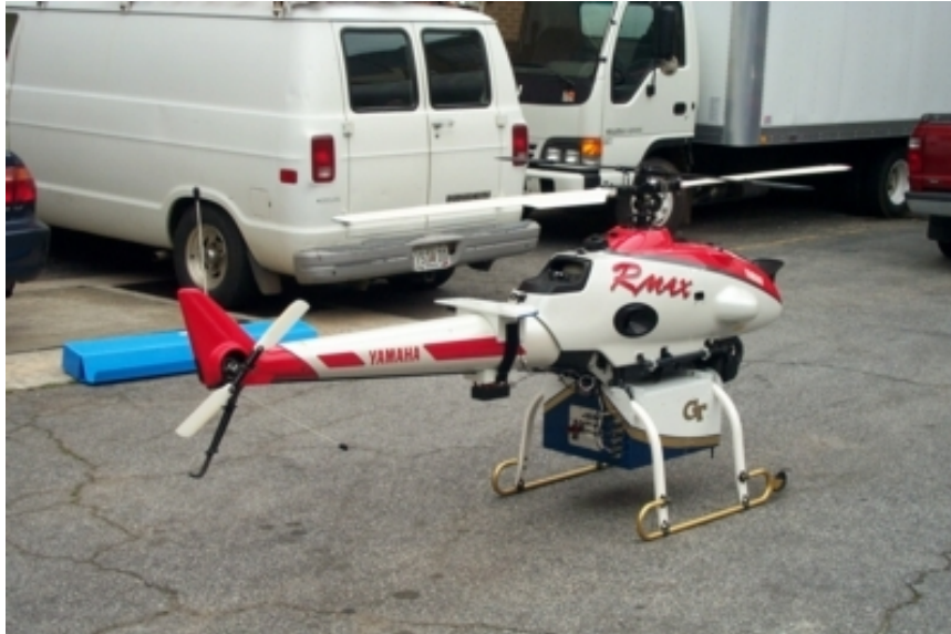
Figure 5: R-Max UAV with main avionics box and boom mount
