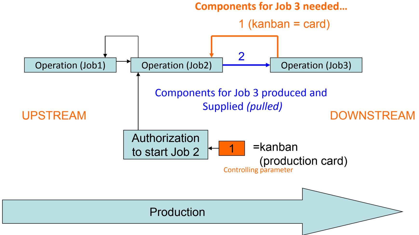
The number of cards in the system determines the WIP levels in the plant
