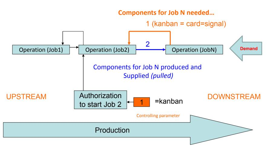
The number of kanban cards in the system determines the WIP levels in the plant
