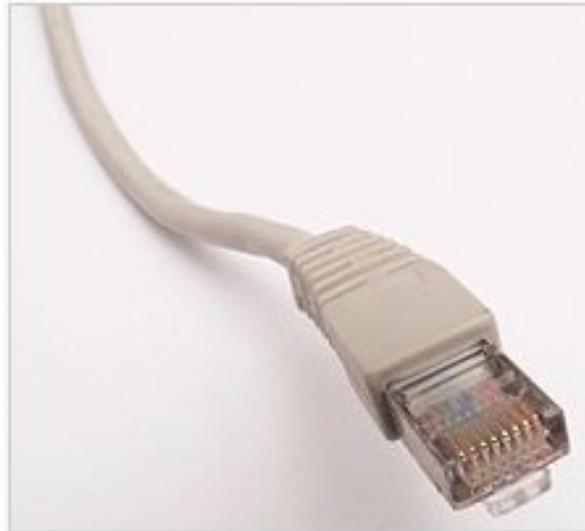
Poka-yoke example: Ethernet cable plug is designed to be plugged in only one orientation.
