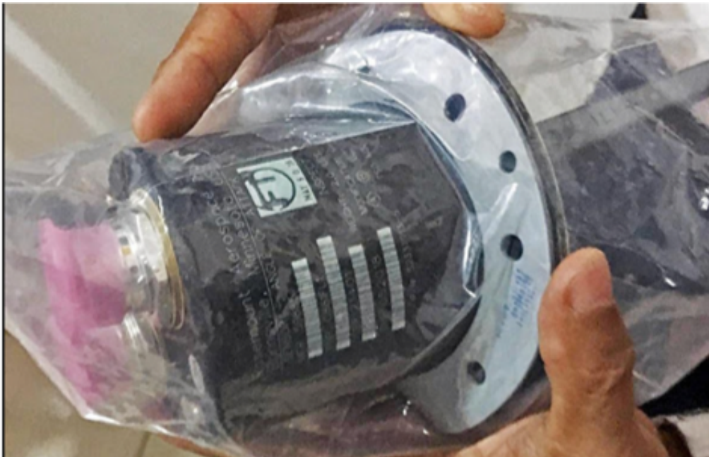
Angle of attack sensor as removed from Lion Air crash aircraft (Timothy McLaughlin/Washington Post)
