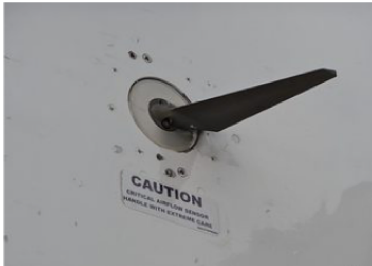
Angle of attack (AOA) sensor
