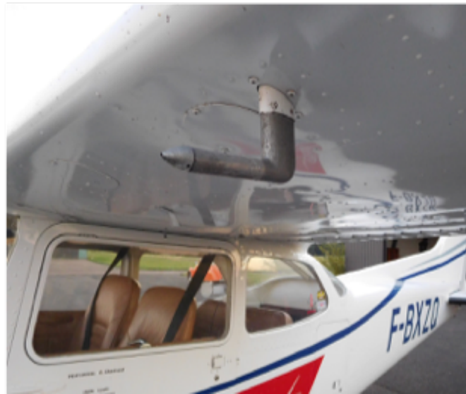
Pitot tubes on a Cessna 172. They look almost exactly the same on a 737.
