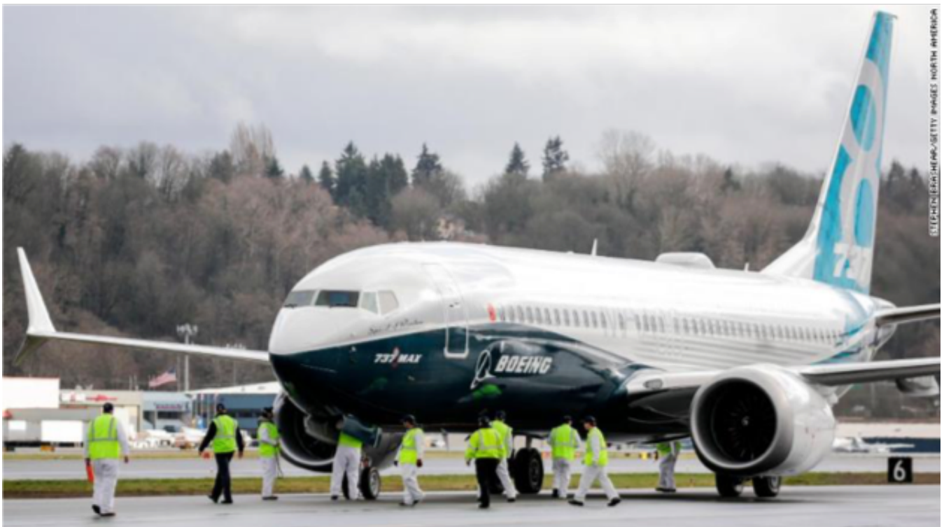
737 MAX. Note size of engines and placement compared to original 737 above. Ca. 2016 (Boeing)
