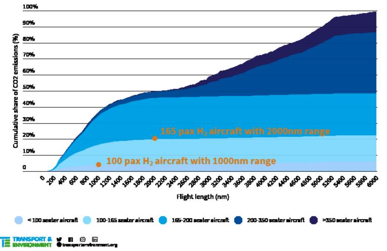
But the real challenge, as so often for hydrogen technologies, is cost. Plane designs would need to be adjusted; bulky hydrogen storage tanks added; and refueling and storage infrastructure created around airports. Fuel costs, which make up around 40% of aircraft operating costs, would also be higher. A 165 seater H2 aircraft would still cost 14% to 33% more than an aircraft running on conventional kerosene. And that's without counting any of the development or hydrogen supply chain costs.
