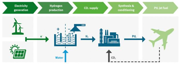
The alternative fuel produced through this process is drop-in compatible and, if produced through the Fischer-Tropsch conversion process, it is already approved for use in aircraft by the ASTM (American Society for Testing and Materials, is an international <u>standards organization</u> that develops and publishes voluntary consensus technical <u>standards</u> for a wide range of materials, products, systems, and <u>services</u>.).
