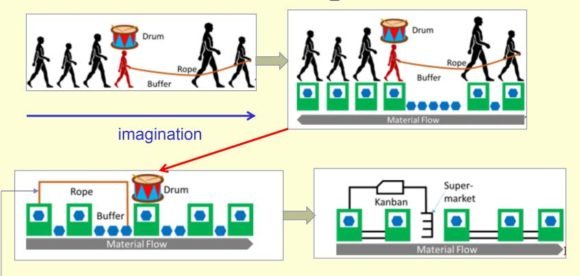
**Feedback** - if the amount of materials in the buffer drops below a certain limit, the input of components to the line is released
