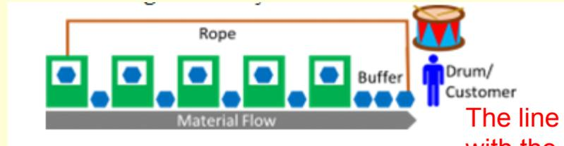
The line is not controlled by the source with the lowest flow (throughput), but by the requirements of the Customers
