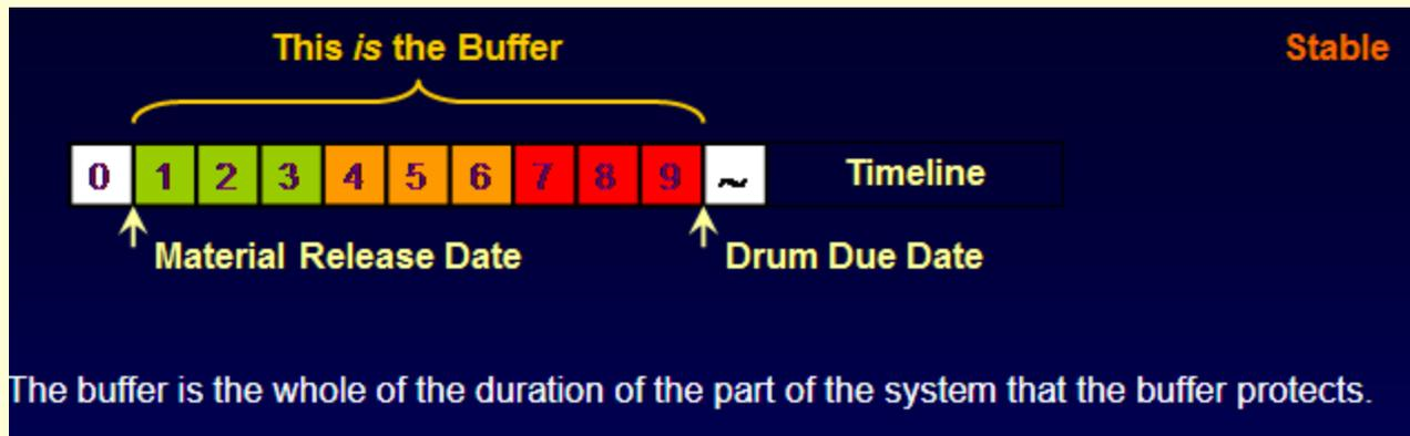
The order of priority for processing parts assigned to different Work Orders is determined by color (as in traffic lights)
