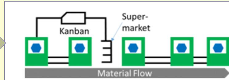
**Feedback** - if the amount of materials in the buffer drops below a certain limit, the input of components to the line is released
