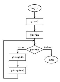
$$\begin{array}{l} \varphi \equiv x1 \geq 0 \ \land \ x2 > 0 \\ \psi \equiv (x1 = y1 * x2 + y2) \ \land \\ \land \ y2 \geq 0 \ \land \ y2 < x2 \end{array}$$
