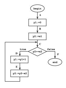
$$\begin{array}{l} \text{initial condition} \\ \varphi \equiv x1 \geq 0 \ \land \ x2 > 0 \\ \varphi_A \equiv \varphi \\ \varphi_B \equiv x1 \geq 0 \ \land \ x2 > 0 \\ \varphi_C \equiv x2 > 0 \ \land \ y2 \geq 2 \\ \varphi_D \equiv x2 > 0 \ \land \ y2 \geq x2 \\ \varphi_E \equiv x2 > 0 \ \land \ y2 \geq x2 \\ \varphi_F \equiv \ y2 \geq 0 \\ e_A = x1 \\ e_B = x1 \\ e_C = \ y2 \\ e_D = \ y2 \\ e_E = \ y2 \\ e_F = \ y2 \\ \end{array}$$
