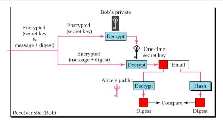
Figure: The mechanism of decrypting and verifying the received message (receiver's side).
