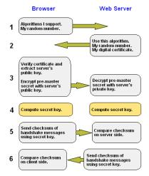
Figure: The SSL handshake (steps 5 and 6 verify the integrity of the handshake; the communication is encrypted using a symmetric (session) key).
