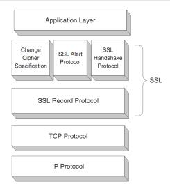
Figure: The SSL protocol stack.
