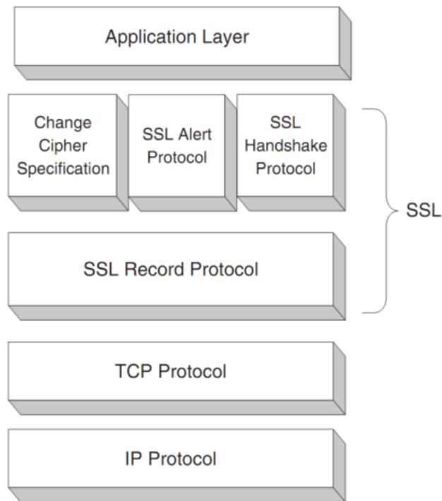
Figure: The SSL protocol stack.
