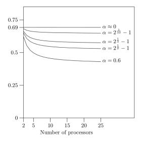
$(m\beta' + 1)(2^{1/\beta'} - 1)/m$  (vertical axis) w.r.t. the number of processors *m*, here  $\alpha = \max_i u_i$  is the maximum utilization
