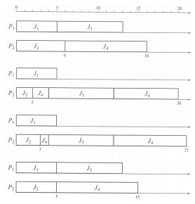
EDF on *m* identical processors: At any time instant, jobs with the earliest absolute deadlines are executed on available processors (Recall: no job can be executed on more than one processor at a given time!)
