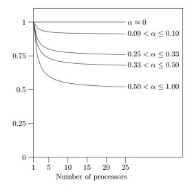
The value  $\left(\frac{\beta m+1}{\beta+1} / m\right)$  (vertical axis) w.r.t. the number of processors *m* (horizontal axis), here  $\alpha = \max_i u_i$  is the maximum utilization
