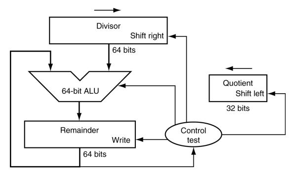
Calculate A = 50 divided by B = 23 using the hardware described below. You should show the contents of each register on each step. Assume A and B are octal unsigned 6-bit integers (adjust the register sizes in the hardware).
