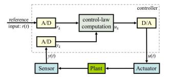
The controller (computer) controls the plant using the actuator (valve) based on sampled data from the sensor (flow meter)
