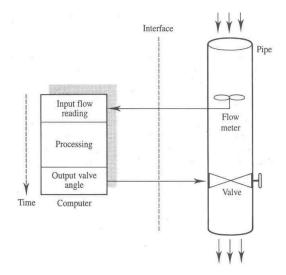
Computer controls the flow in the pipe in real-time
