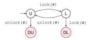
U = unlocked error states: DU = double unlock
