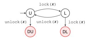
U = unlocked L = locked error states: DU = double unlock DL = double lock
