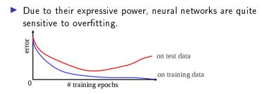
Keep a hold-out validation set and test accuracy on it after every epoch. Stop training when additional epochs actually increase the validation error.
