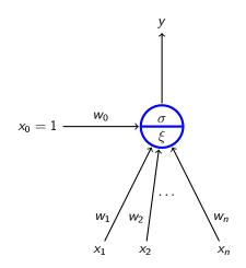
x<sub>1</sub>,..., x<sub>n</sub> real *inputs* x<sub>0</sub> special input, always 1
