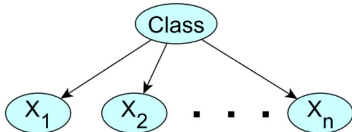
$$P(C, X_1, \dots, X_n) = P(C) \prod_{i=1}^n P(X_i|C)$$
