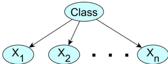
$$\frac{P(C=c^1|x_1, \dots, x_n)}{P(C=c^2|x_1, \dots, x_n)} = \frac{P(C=c^1)}{P(C=c^2)} \prod_{i=1}^n \frac{P(x_i|C=c^1)}{P(x_i|C=c^2)}$$
