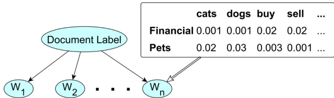
$$\frac{P(C=c^1|x_1, \dots, x_n)}{P(C=c^2|x_1, \dots, x_n)} = \frac{P(C=c^1)}{P(C=c^2)} \prod_{i=1}^n \frac{P(x_i|C=c^1)}{P(x_i|C=c^2)}$$
