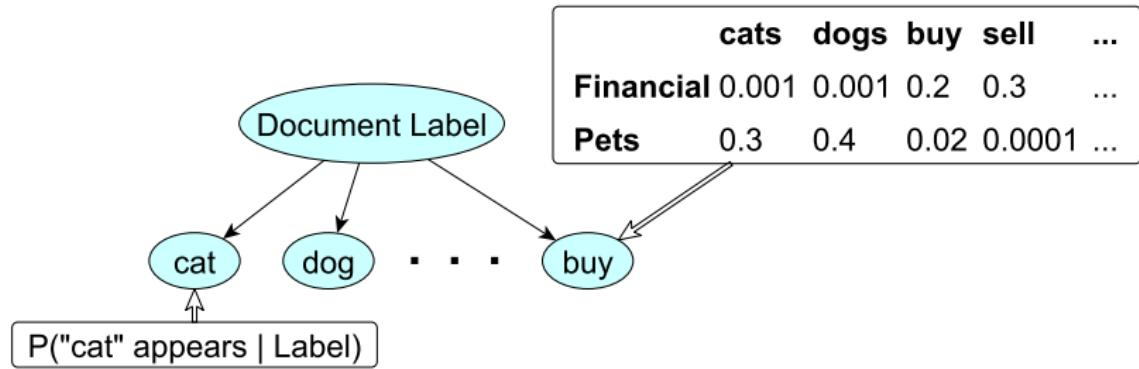
$$\frac{P(C=c^1|x_1, \dots, x_n)}{P(C=c^2|x_1, \dots, x_n)} = \frac{P(C=c^1)}{P(C=c^2)} \prod_{i=1}^n \frac{P(x_i|C=c^1)}{P(x_i|C=c^2)}$$
