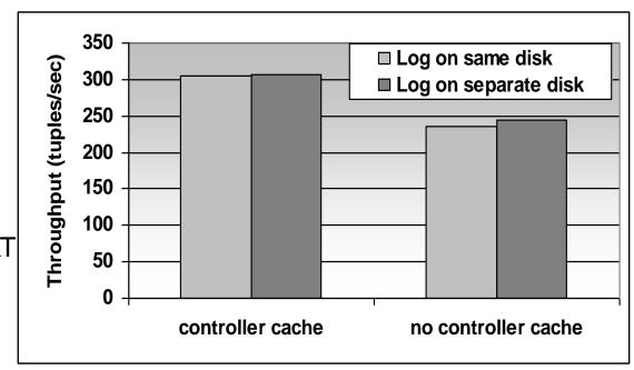
Controller Cache diminishes negative impact of non-dedicated disk HW: middle server, Adaptec RAID controller (80Mb RAM), 2x18Gb disk.
