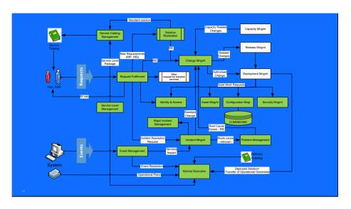
ITSM tool functionality does not need to cover all 100% framework processes/functions. Here is the example how some of processes are covered by the new tool (green) and some vere left in old solution (white). The important here is to assure reliable and correct linkage between those two solutions.
