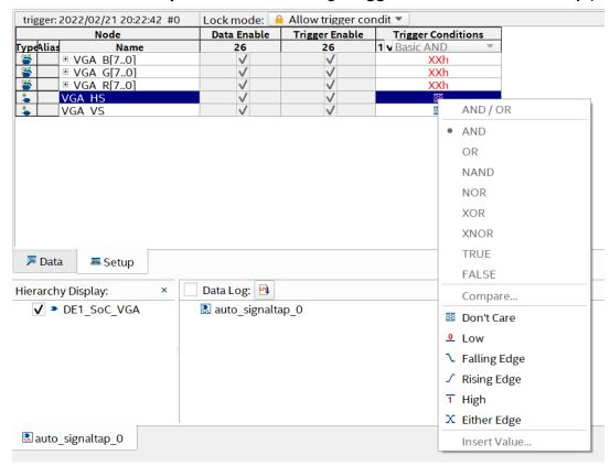
When you are done with debugging, do not forget to get rid of the files the analyzer inserted into your project! It slows the compilation down considerably and uses valuable FPGA resources. In the Quartus project settings (Assignments -> Settings):
