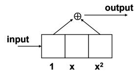
will multiply the input stream by x<sup>2</sup>+1 and the second shift register
