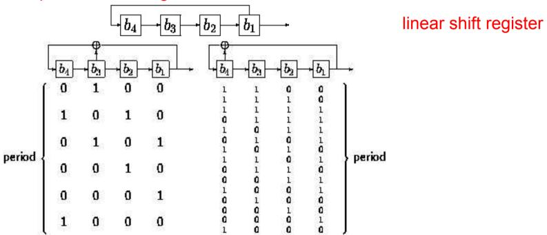
Theorem For every n > 0 there is a linear shift register of maximal period  $2^n - 1$ .
