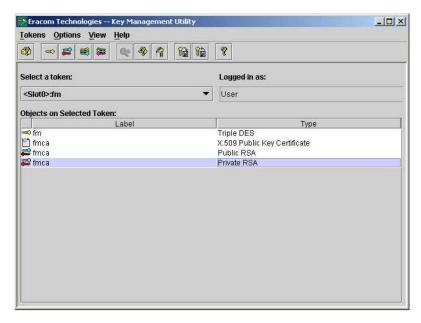
Once a token has been selected the user will be given the option to login. After the PIN is successfully authenticated, a list of keys and other objects contained within the token is displayed in the "Objects on Selected Token" box. Appropriate buttons on the toolbar will now also be enabled as shown on the picture.
