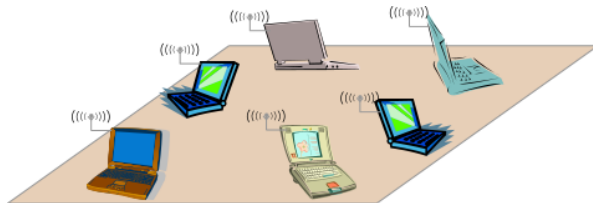
Figure: Simple example: laptops in a conference room – a single-hop ad-hoc network (all the networking nodes are in a direct communication range of each other node).
