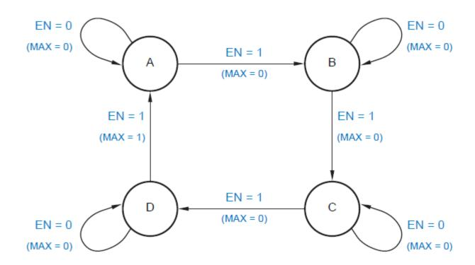
• In state diagram for a **Moore machine**, output values can be shown inside each state circle, since they are functions of state only.
