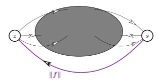
• simply add the "reverse" arc (s,z) assigned flow value ||f|| and capacity  $+\infty$ .
