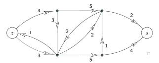
Remark: In a real world, more than one source or sink may exist in a flow network, but that is not a problem—we simply create a single artificial "supersource" and draw arcs from it to all the real sources (even with source capacities), and the same with a "supersink".
