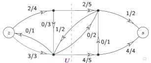
**Fact**: The boundary surplus of f on  $\{z\}$  is exactly the flow size ||f|| by the definition. We aim to extend this finding to other suitable U's.
