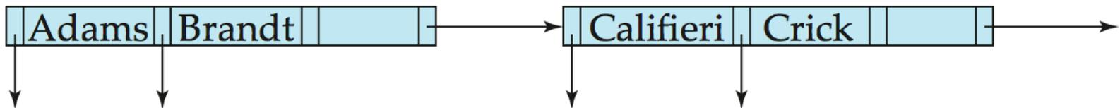
Result of splitting node containing Brandt, Califieri and Crick on inserting Adams
