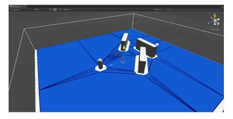
Fig. 3.9.4.: Navigation mesh generated around the "First Person Controller" (the capsule)
