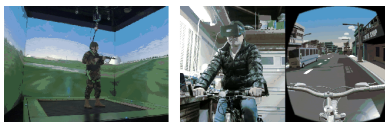
(a) An omnidirectional treadmill used in a CAVE system by the US Army for training. (b) A home-brew bicycle riding system connected to a VR headset, developed by Paul Dyan
