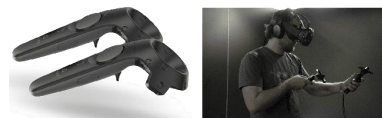
(a) A pair of hand-held controllers that came with the HTC Vive headset in 2016; the device includes side buttons, a trigger, and a touch pad for the thumb. (b) A user trying the controllers (prototype version)
