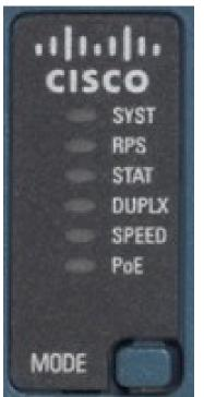
**System LED (SYST):** Shows whether the system is receiving power and functioning properly.
