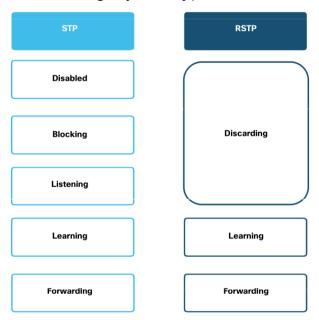
Root ports and designated ports are the same for both STP and RSTP. However, there are two RSTP port roles that correspond to the blocking state of STP. In STP, a blocked port is defined as not being the designated or root port. RSTP has two port roles for this purpose.
