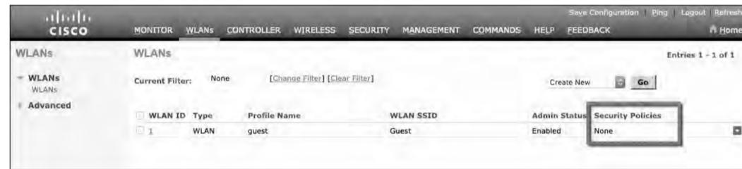
**Figure 20-4** Verifying Open Authentication from List of WLANs
