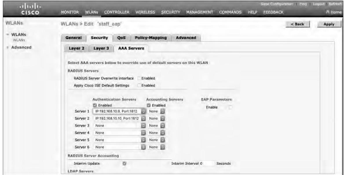
**Figure 20-11** *Selecting RADIUS Servers to Authenticate Clients in the WLAN*
