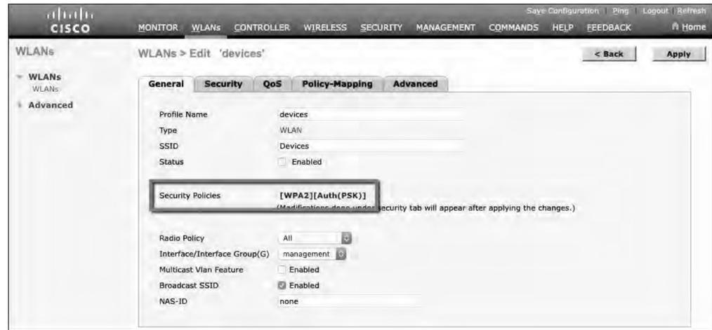
Figure 20-6 Verifying PSK Authentication in the WLAN Configuration
