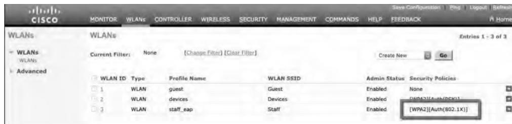
Figure 20-17 Verifying EAP Authentication on a WLAN
