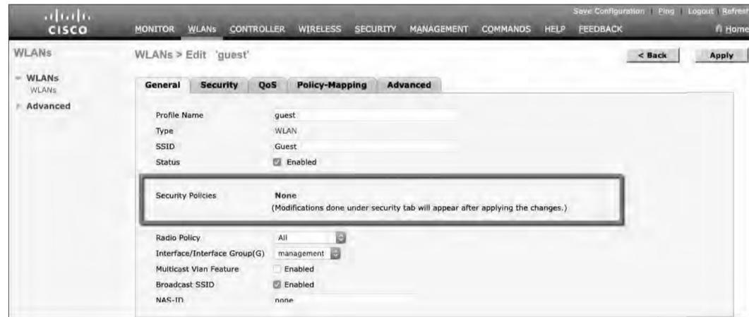
**Figure 20-3** Verifying Open Authentication in the WLAN Configuration
