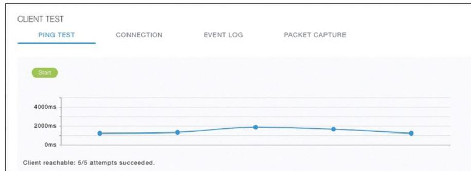
**Figure 21-9** Testing Ping Response Times Between the WLC and Client
