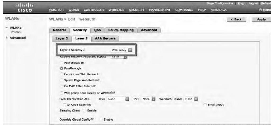
Figure 20-19 Configuring WebAuth with Passthrough Authentication
