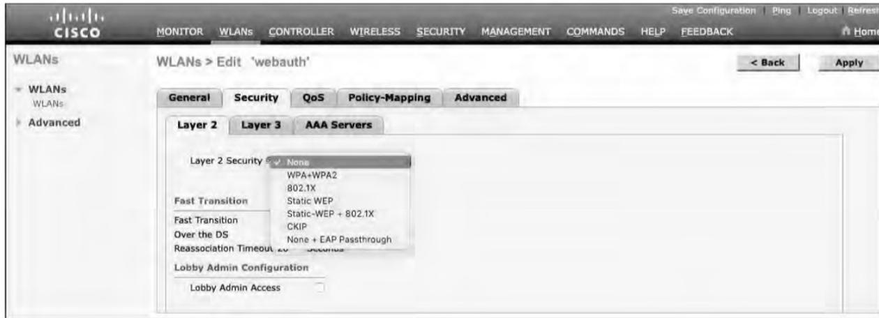
In Figure 20-18, the WLAN is named webauth, the SSID is Guest\_webauth, and Open Authentication will be used because the None method has been selected.
