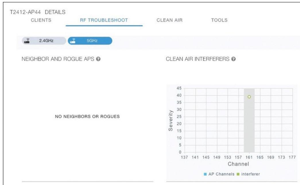
Figure 21-16 Displaying Information About RF Interferers
