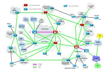
Figure: The topology of the  $\mathsf{IP}/\mathsf{MPLS}$  layer of the CESNET2 network.
