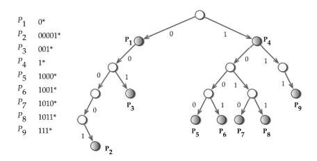
Figure: Binary trie data structure example.
