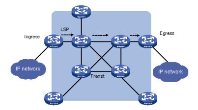
Figure: Structure of the MPLS network.
