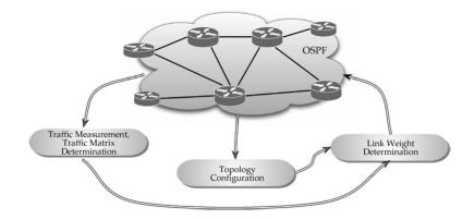
Figure: IP Traffic Engineering architectural framework.
