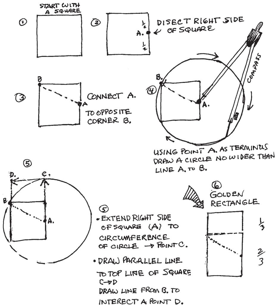
Figure 4-2 Follow the simple steps indicated in this schematic drawing to construct a golden rectangle (divine proportion).
