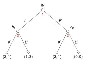
Here  $h_0,h_1,h_2$  are non-terminal nodes, leaves are terminal nodes. Each non-terminal node is owned by a player who chooses an action. E.g.,  $h_1$  is owned by player 2 who chooses either K or U Every action results in a transition to a new node. Choosing L in  $h_0$  results in a move to  $h_1$
