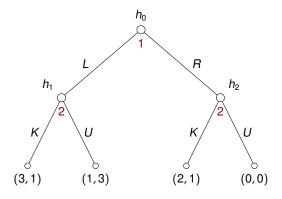
Here  $h_0$ ,  $h_1$ ,  $h_2$  are non-terminal nodes, leaves are terminal nodes.
